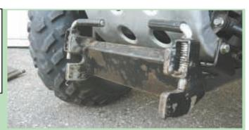
Quick-tach front hitch bolts to protection plate on ATV.
