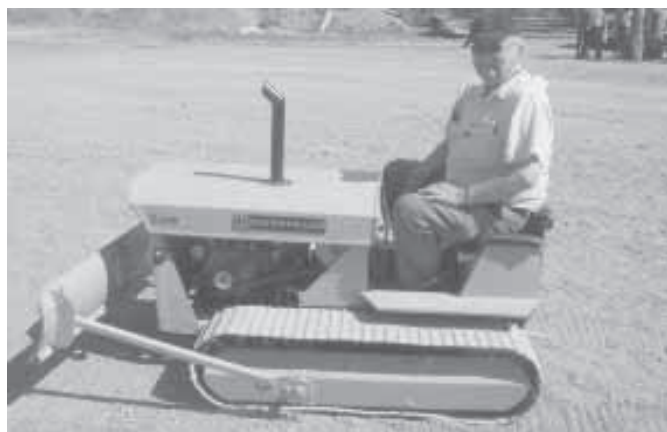
"I worked on it for about a year and rebuilt it several times to get it right," says Jim Golly, who built this Cat D8 mini dozer without a pattern.
