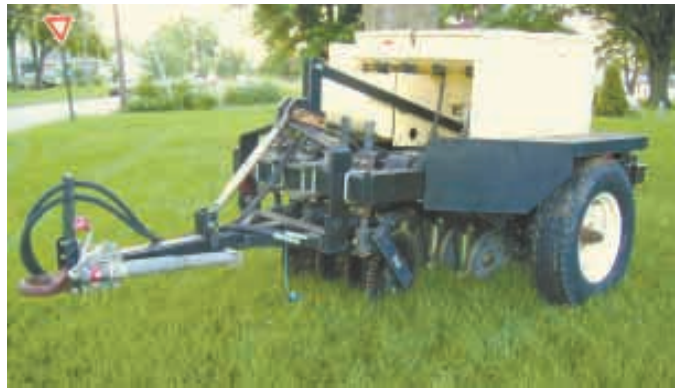
Dew Drop Drill is designed to "solid seed" crops rather than plant in rows.
