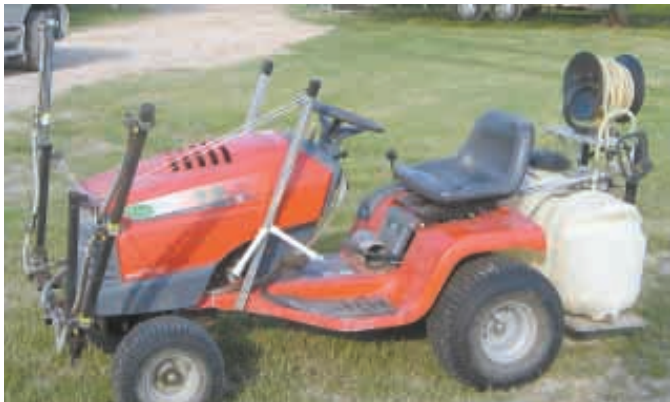
With a front-mounted boom and rear-mounted hand nozzle with 50 ft. of hose, Karl Cole can do many different kinds of spray jobs around his farm.
