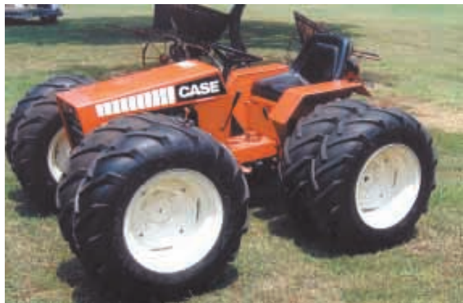
"It's definitely unique," says Gary Pyron, who mounted eight 8 by 16 tires on his 16 hp Case 446 garden tractor.
