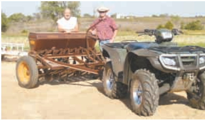
Kenneth Hill had friend Andy Fenley cut an old Minneapolis Moline 14-ft. end wheel drill in half to build this 6-ft. 8-in. wide drill. He pulls it with an ATV or small tractor.
