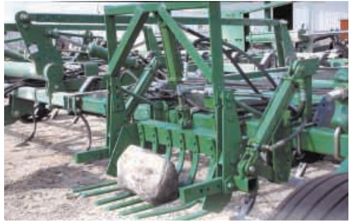
Bolt-on rock lifter attaches to field cultivator and is operated by three hydraulic cylinders. Two cylinders raise or lower the basket, and one dumps.
