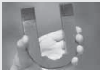
Spring Spacers are inserted into springs to increase down pressure on openers. Photo below shows spacer installed.
