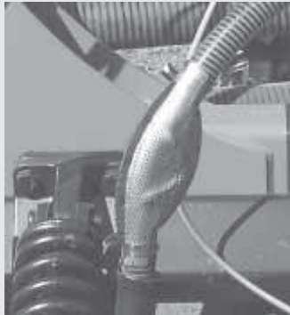
Installed above the seed boot, the Seed Brake is a perforated stainless steel tube. It allows most of the air to dissipate, which keeps the seed from being blown out of the seed slot.
