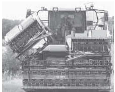
Geringhoff's new folding grain header folds to about 12 ft. wide.
