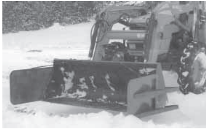
Snow boards, shown here in retracted position, almost double bucket width when in extended (plowing) position. Bungee cords hold boards in when not in use.
