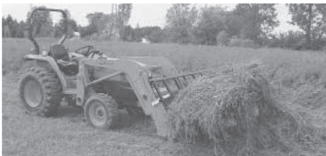
Buckrake attaches to the front-end loader on Dykstra’s Kubota tractor.
