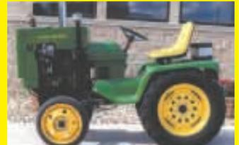
I always wanted a garden tractor equipped with a Deere 2-cyl. engine, so recently I mounted an LUC engine off a Deere 12-A combine in a Deere 318 garden tractor. It's chain-driven and has a hydrostatic transmission. (*Norman Kielsmeier, Rudd, Iowa 50471 ph 641 395-2668*)
