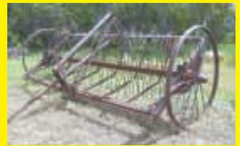
never seen one like it. The rake was originally made to be pulled by horses, but someone added a hitch to pull it behind a tractor. When it was new it probably had a seat and caster wheels on front.
