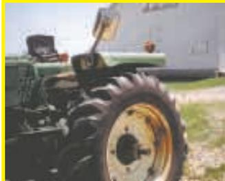
I mounted a truck mirror on the leading edge of the rear fender on my tractor. It helps me see around towed wagons. That's especially handy on the highway. (*Al Doering, 19828 310th St., Hubbard, Iowa 50122 ph 641-864-3554*)
