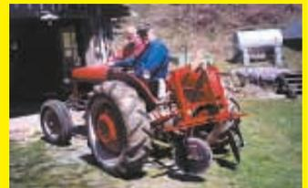
I built this 3-pt. mounted "lay-off plow" to plant potatoes in my garden and use my 1950 Ferguson 85 hp tractor to pull it. The unit consists of two 16-in. dia. discs mounted on a frame that's made from 3/8-in. thick, 2 1/2-in. angle iron. The discs are spaced 1 1/2 ft. apart and hill up the soil about 6 in. high.
