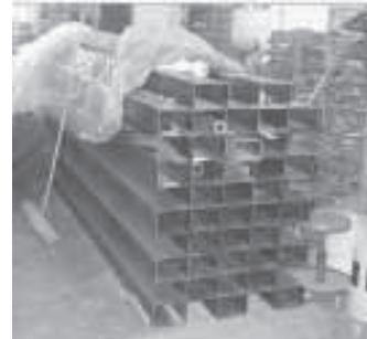
Compartments each measure 5 by 7 in. and are set up in a "checkerboard" pattern, to reduce the amount of tubing needed.
