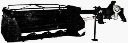
Individual discs have 3 reversible blades and operate at 3,000 rpm, allowing them to cut through wet, heavy and tangled crops at high speeds.
