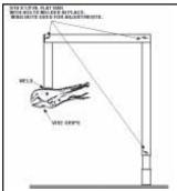
lot of welding of small parts and sometimes I need a third or fourth hand. That's why I made this 'third hand' device from a locking pliers and scrap metal. Sure works well. I made it out of 3/16 by 1/2-in. flat bar, with bolts welded into each hinge point with hand-tightened wing nuts."
