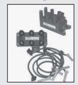
Screamin' Demon coil allows you to open plug gaps to .065. The largergap creates a hotter, longer duration spark.
