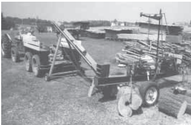
One of the newest components in James Goetsch's firewood cutting and splitting system is a conveyor that's used to deliver firewood into a trailer.
