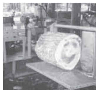
Side-mounted hydraulic lift lifts wood and rolls it onto splitting platform.
