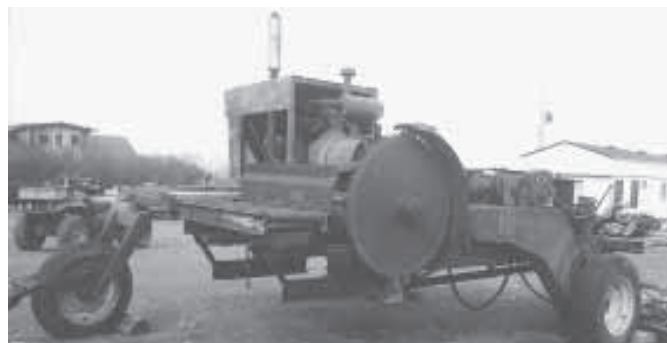
Using an old swather and the leg off an old road grader, Jim Rife made this mobile wood splitter-buzz saw combination unit.
