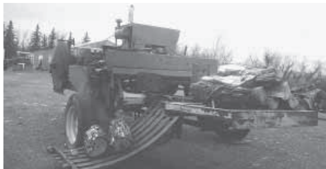
Side-mounted hydraulic lift lifts wood and rolls it onto splitting platform.
