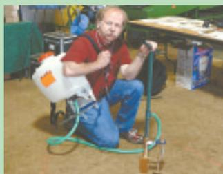
The Yoder backpack transplant tool is a neat alternative to the expensive pull-type equipment used by large market gardening and produce growers. The hand tool is designed to open a space by pushing down on loose soil. The spade opens, and liquid fertilizer is delivered into the hole. The operator then drops a starter plant into the hole and tamps the dirt down around it.
