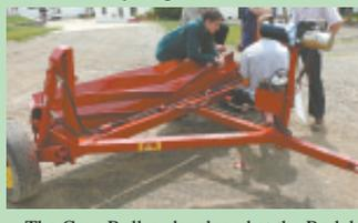
The Crop Roller, developed at the Rodale Institute and now being built by I&J Mfg., lays down and chops up crop residue, cover crops, or old hay crops prior to no-till or zone-till planting. The mat of residue it leaves on the ground holds down weeds. Units start at \$2,800.
