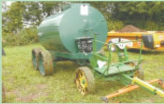
This 1,000-gal. liquid manure spreader from ELS sells for \$3,870 with ground or pto drive and is equipped with a gravity baffle. Other sizes range from 600 to 1,600 gal.
