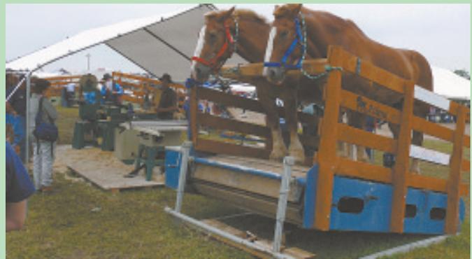
Horse-powered treadmills are equipped with pto gearboxes and can be used to power everything from metal and wood working equipment to grain mills and water pumps.
