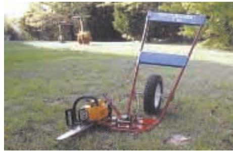
With the tug of a rope, chainsaw bar can be positioned horizontally or vertically.
