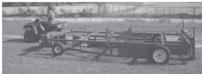
No-hydraulic bale accumulator uses a series of levers to guide bales into four chambers as accumulator is pulled through field (above). It can be pulled with equipment as small as a pickup or ATV, or hooked up directly behind a small square baler.
