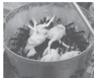
Equipment includes a 42-gal. rotary scalding and 27-in. drum picker.
