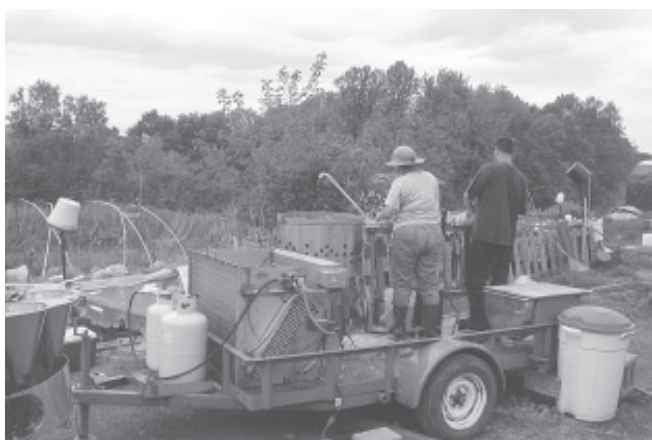
Poultry processing equipment is carried on a 6 by 12-ft. road-legal trailer.
