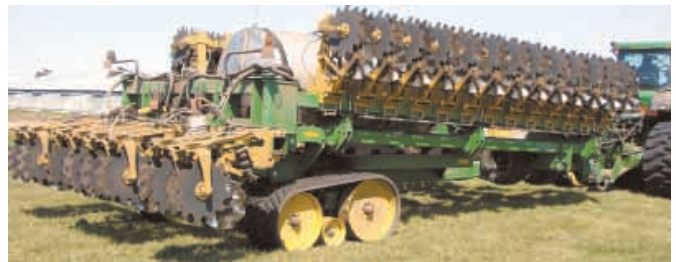
Hermanson's 60-ft. Houck bar is carried by 24-in. wide tracks. He pulls it with a Deere 9400T at speeds ranging from 7 to 9 mph.
