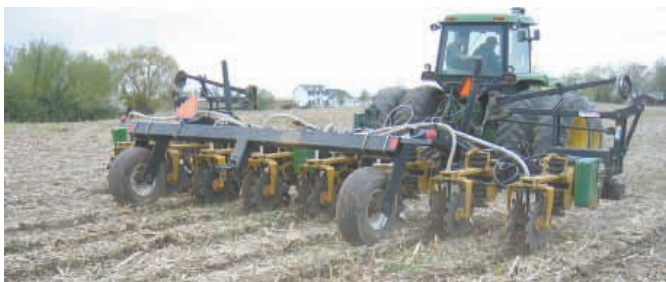
Near Lodi, Wis., 8 Mini-Warrior strip-tillage units were mounted on a 24-ft. Yetter toolbar by Ronnie and James Treinen.
