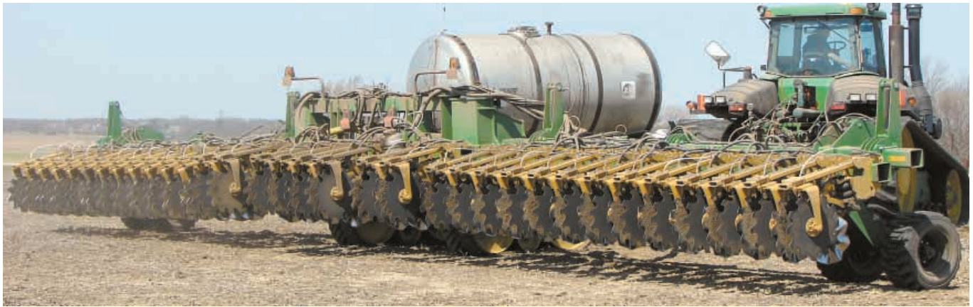
Mike Hermanson, Story City, Iowa, mounted 34 of the new Mini-Warrior™ strip-till row units on 20-in. centers on a 60-ft. folding toolbar.
