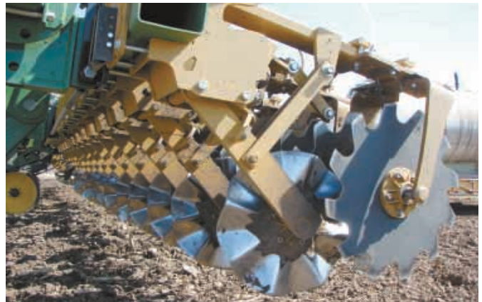
Strip-tillage row units from Environmental Tillage systems have a single 24-in., 8-wave coulters followed by two saber-tooth containment coulters. There's no shank or conventional row cleaners. A unique air spring system provides down pressure.
