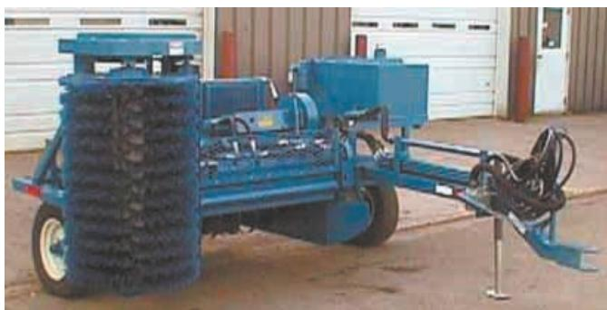
Vertical street sweeper-type bristles pick up weeds and debris and kick it over to the machine, which uses double-edge knives to chop the material up fine.
