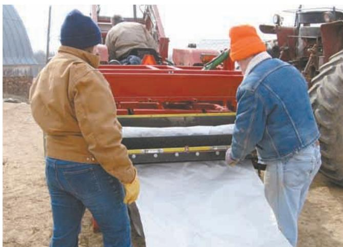
Prototype silo-bag washer may one day help farmers dispose of plastic used for silage bags and bunker covers. It brushes dirt off the plastic, pulls the plastic through rollers and deposits it in a basket where it's compacted with a plunger, ready to be tied into a plastic bale about the size of a small hay bale. The machine operates off tractor hydraulics.
