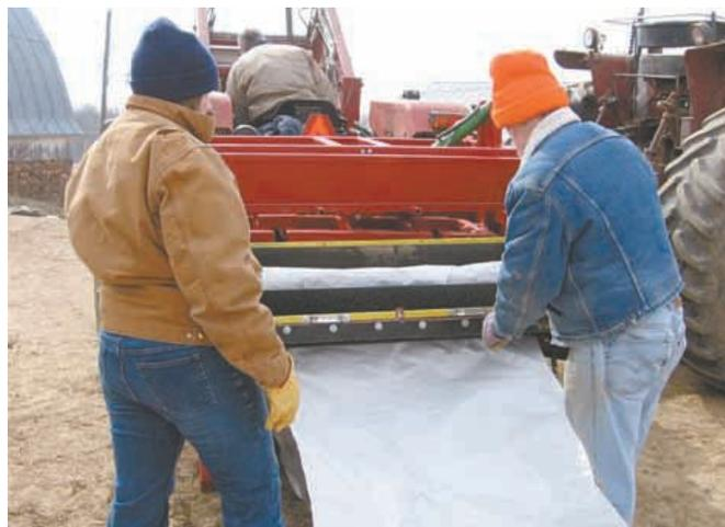
Prototype silo-bag washer may one day help farmers dispose of plastic used for silage bags and bunker covers. It brushes dirt off the plastic, pulls the plastic through rollers and deposits it in a basket where it's compacted with a plunger, ready to be tied into a plastic bale about the size of a small hay bale. The machine operates off tractor hydraulics.
