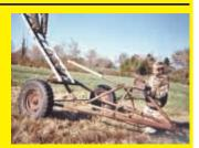
To use my 20-ft. ladder to cut branches safely, I mounted it on an old auger elevator I had laying around. The ladder bolts to the steel boom. It can't get loose. Then I attached a winch to the auger's frame and ran a 1/4-in. steel cable from it to the boom. It easily pulls the ladder and boom up to different angles.
