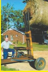
I use the machine to haul bales from the field to my barn and also to stack them. It's equipped with a spear on back and will lift bales up to 12 ft. high. The top part of the spear pins onto the mast while the bottom part clamps on. A big advantage of this design is that it keeps all the bale's weight off my tractor.
