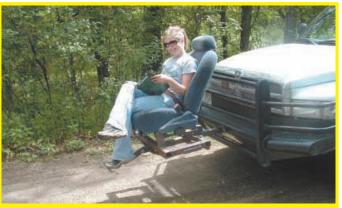
Here's a photo of what I call my "Cass County Deer Stand". It's a bucket seat from a Chevy Cavalier welded onto a metal frame that fits into a 2-in. receiver hitch on front of a vehicle. I built it mainly for entertainment, but it has proven useful here at the U.S. Army's Camp Ripley in Minnesota.
