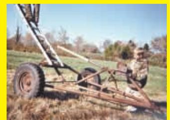
To use my 20-ft. ladder to cut branches safely, I mounted it on an old auger elevator I had laying around. The ladder bolts to the steel boom. It can't get loose. Then I attached a winch to the auger's frame and ran a 1/4-in. steel cable from it to the boom. It easily pulls the ladder and boom up to different angles.
