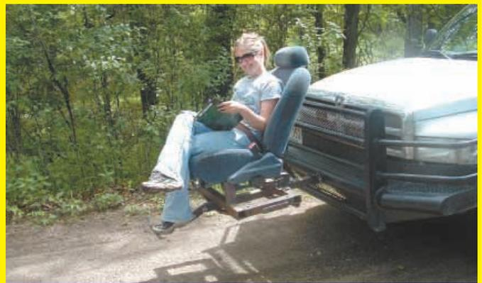
Here's a photo of what I call my "Cass County Deer Stand". It's a bucket seat from a Chevy Cavalier welded onto a metal frame that fits into a 2-in. receiver hitch on front of a vehicle. I built it mainly for entertainment, but it has proven useful here at the U.S. Army's Camp Ripley in Minnesota.
