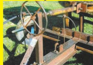
A big wheel mounts above the tongue and is used to tilt the mast in order to keep the bale from falling off the spear. After raising the bale off the ground, I get off the tractor and turn the wheel about 10 times to tilt the mast six degrees forward. I'd like to use a hydraulic cylinder to tilt the mast so I wouldn't have to get off the tractor, but my tractor doesn't have dual hydraulic outlets.
