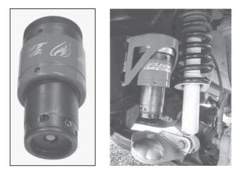
Designed for full-size pickups, the JounceShock supplements a vehicle's existing shocks.
