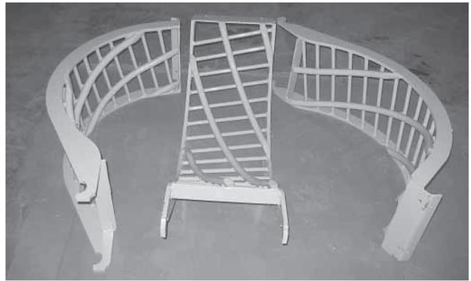
Heavy duty steel concave for Case IH combines is designed to do a better job of removing chaff and cleaning grain with less damage and cracking.
