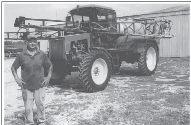
Gale Courson, Farina, Ill., converted an IH school bus into this 70-ft. boom sprayer. The original bus had a 6-cyl. engine and 4-speed transmission. He changed the rear end to a 2-speed low range job. He built the front axle and the hood. The axle was built from 5-in. steel tubing. The rear tires are 14.9 by 46; front 14.9 by 44. An inflatable truck spring is built into the boom to reduce shock on the boom.
