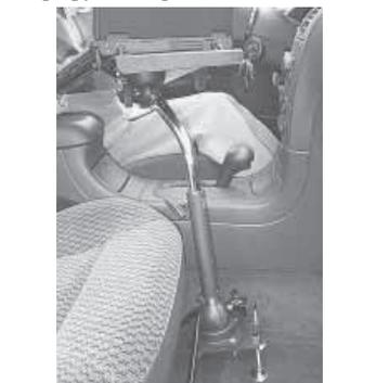
Telescoping pedestal supports computer and mounts on a ball joint swivel mechanism that attaches to base.
