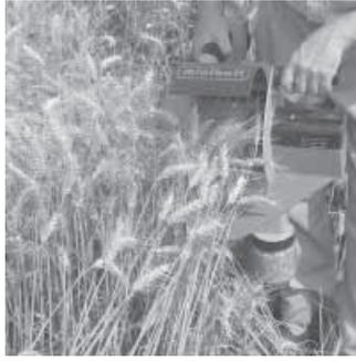
Handheld unit operates like a mini combine, harvesting and threshing small grain at a rate of about 3 1/2 oz./min.
