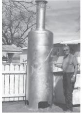
Wayne Hardenbergh built this incinerator out of an old 250-gal. butane tank
