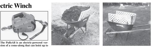
"Expander" consists of 12-in. high lattice-type pvc panels that attach to wheelbarrow sides with wing nuts. Works well to haul bulky materials like leaves or lawn clippings.
