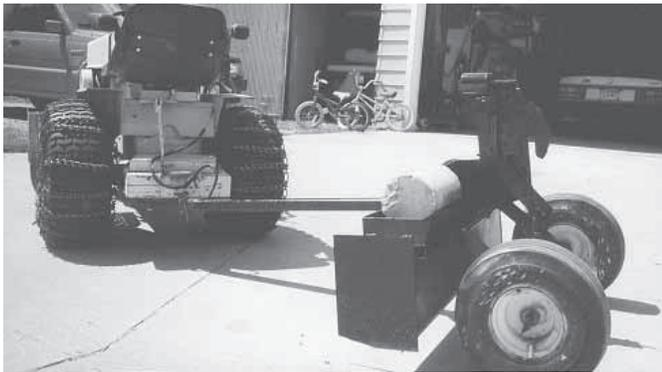
An electric window motor is used to raise and lower the grader on-the-go.
