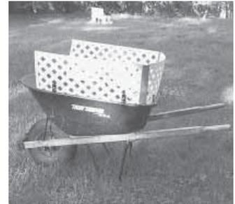
"Expander" consists of 12-in. high lattice-type pvc panels that attach to wheelbarrow sides with wing nuts. Works well to haul bulky materials like leaves or lawn clippings.
