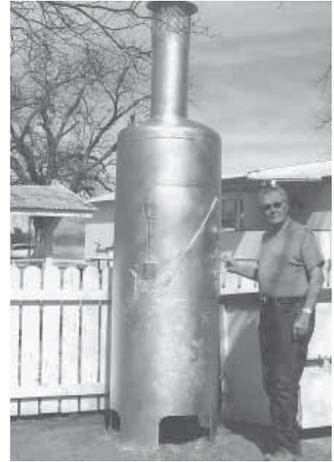
Wayne Hardenbergh built this incinerator out of an old 250-gal. butane tank
