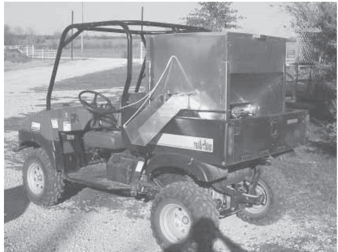
Self-contained "feeder box" uses an electric motor to chain-drive an auger that delivers feed from a side-unloading spout.
