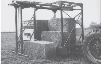
Hydraulic-powered carriage on top of channel iron frame raises and lowers bale lift mechanism, which picks bales off the field and moves them onto a bed.
