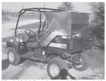
Self-contained "feeder box" uses an electric motor to chain-drive an auger that delivers feed from a side-unloading spout.
