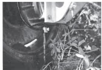
To drain water from gearbox all you have to do is turn a wrench.
