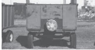
To dry wildflower seeds fast, Andrew Swanson installed a perforated metal false floor in a wagon and mounted an ordinary bin fan in the endgate.
