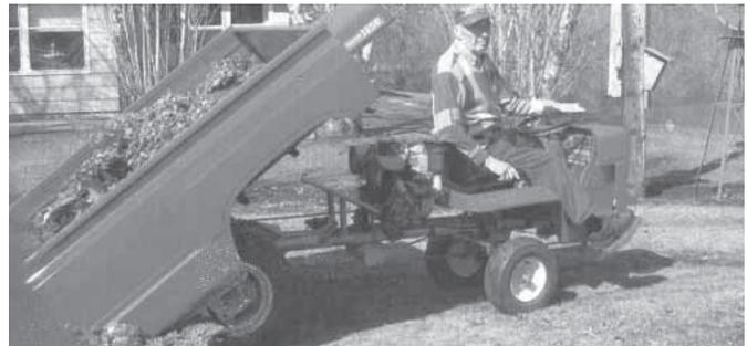
To build a powered dump cart Joe Roller stretched out a Bolens 1256 garden tractor, then mounted an old pickup box on it.
