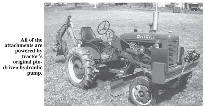
**All of the attachments are powered by tractor's original pto-driven hydraulic pump.**
