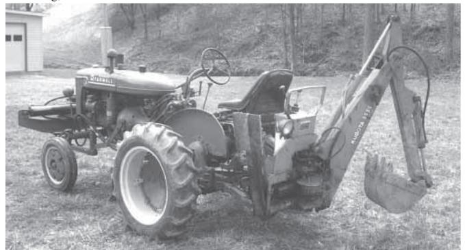
**Reginald Suan fitted this old Farmall A with a hydraulic-operated Kubota backhoe, belly-mount blade, and front-mount log splitter.**
