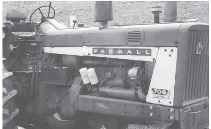
**Brian Tworkoski says converting a gas-powered Farmall 706 to diesel is a snap. All you need is a 400 Series International engine and a clutch and flywheel to match.**
