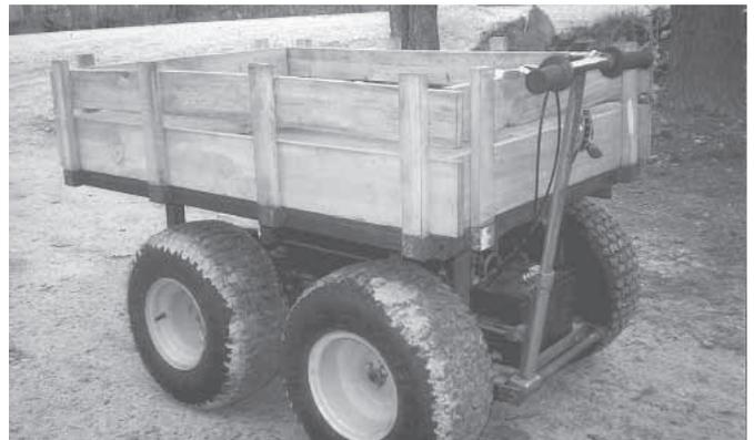
**Dump-style wood hauler is powered by a 10 hp Tecumseh engine. The hydrostatic transaxle drive out of a Cub Cadet garden tractor chain-drives all four wheels.**
