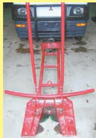
Tree Chopper was originally designed to be mounted to an ATV. Walnofer designed his own frame mount for his truck.
