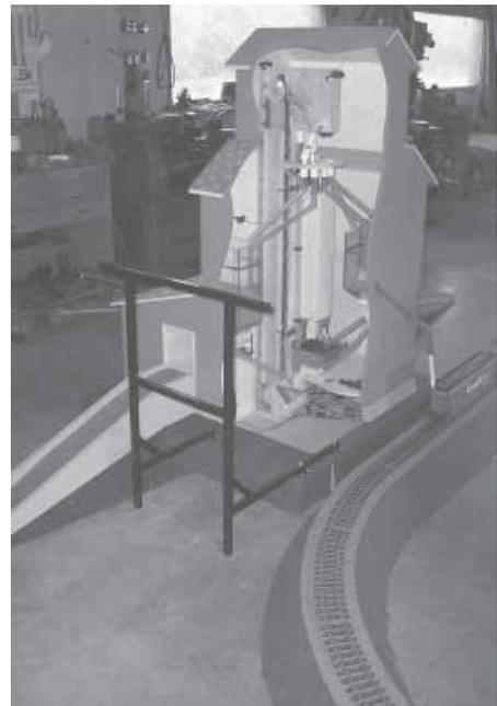
Harvey also built this intricate working model grain elevator, leaving one corner open so people can see how it works. Elevator stands about 5 ft. tall and all operations can be controlled remotely. Grain loads out onto a mini truck or train. Three people at a time are allowed to work the controls. One drives a belly dump truck, one drives the train, and one runs the console on the elevator.
