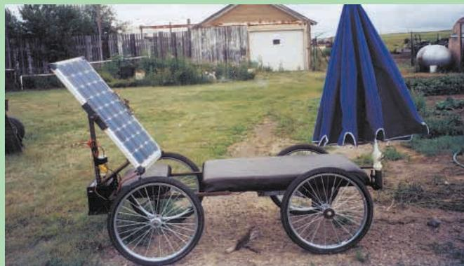
**Garden creeper's 50-watt panel charges a battery that powers a 12-volt motor.**
