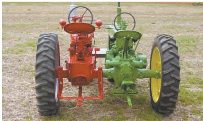
Evans can steer the twinned tractors from either seat, using either engine. He can only power up one of the tractors at a time.
