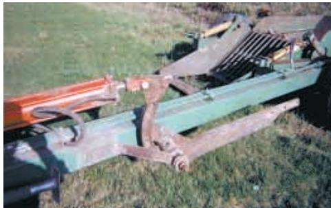
Beam off an old Deere 3-bottom plow is free to pivot and is connected to a hydraulic cylinder that's anchored on rock picker's tongue. "It lets me dislodge rocks that are too deep for the rock picker to pick up," says Juhl.
