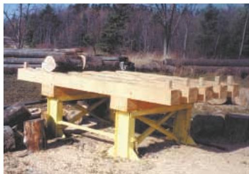
Table is designed so two operators can cut firewood at the same time, one at each end of table, without having to bend over. The operator cuts through log at every space between the timbers.
