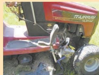
He installed a reversible 12-volt motor to control the steering wheel through a pulley and belt system (left). Another motor controls forward and reverse on the transmission.
