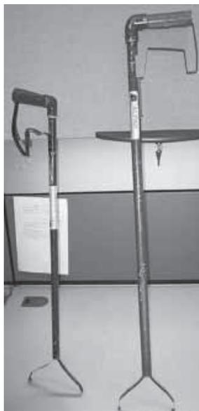
Handheld “garbage grabber” is designed to pick up trash using metal tongs made from recycled flat metal banding.
