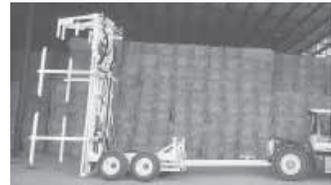
Wagon’s working table has two pivot points - one front and one back.
