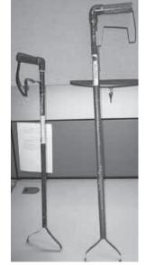
Handheld "garbage grabber" is designed to pick up trash using metal tongs made from recycled flat metal banding.
