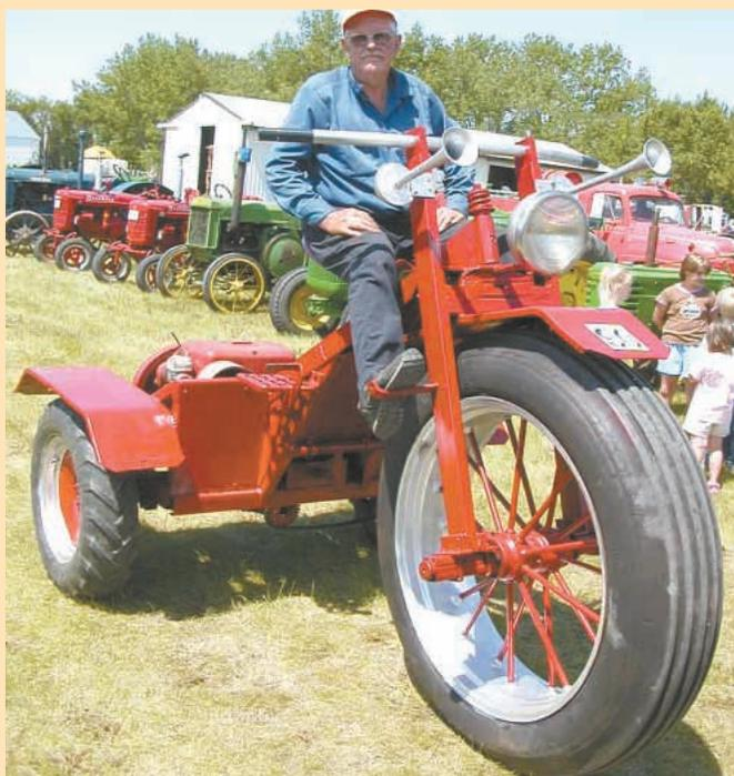
Giant 3-wheeler is a big hit at parades and shows. The big, spoked front wheel has an 11 by 36-in. tire off a 1950's combine. The two small back wheels are off a corn planter.
