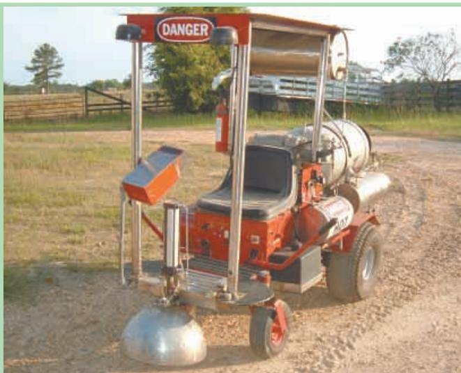
Machine injects 500-degree steam into center of fire ant nests at 40 to 50 lbs. of pressure. The steam kills the queen, which is all it takes to destroy a colony.
