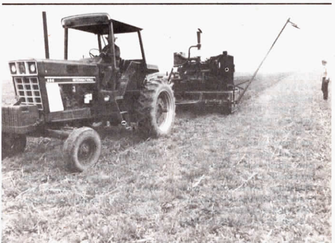
Machine can prepare "one pass" seedbed in stalks or stubble at 4 mph.
