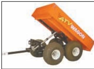
An electric motor gear-drives an electronic screw jack that cranks the bed up or down.
