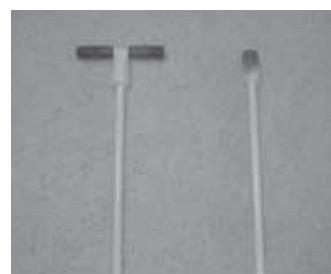
Electric fence post driver is made from a 25-in. length of metal pipe.
