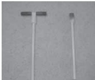
**Electric fence post driver is made from a 25-in. length of metal pipe.**
