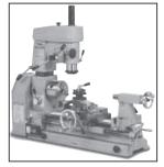
The 3-in-1 "Smithy" combines a mill, drill, and lathe in one machine.
