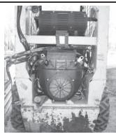
now runs much smoother and quieter and has a lot more power. The new engine came complete with a starter, and the wiring and control cables fit without requiring any alterations. I did run a new wire from the starter to the ignition switch, bypassing the original starter solenoid.
