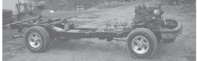
Then he installed the combine engine and new transmission and put the body back in place.
