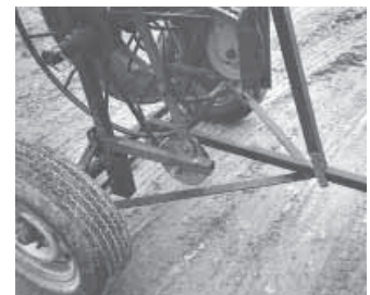
A double V-belt brake is used to adjust tension on reel so wire doesn't unwind too fast and get tangled up.
