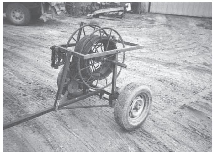
To build wire unroller, Robert Hittle started with the wheels and front spindles off a 1973 Ford Pinto, welding a length of tubing between the spindles to serve as the axle.
