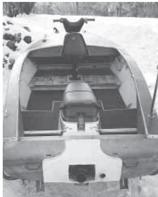
Water jet fits through a hole that Smith cut into back of boat.
