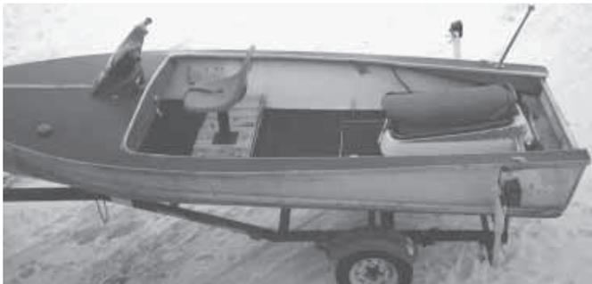
Tim Smith split a 1993 Kawasaki Jet Ski in half, mounting the engine and waterjet at the back of a 14-ft. aluminum speedboat.
