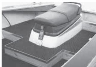
Back half of Jet Ski mounts on an elevated platform at rear of boat.
