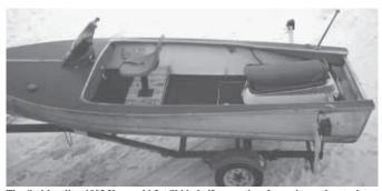
Tim Smith split a 1993 Kawasaki Jet Ski in half, mounting the engine and waterjet at the back of a 14-ft. aluminum speedboat.
