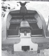
Water jet fits through a hole that Smith cut into back of boat.
