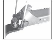
Coupler is fitted with a pair of vertical fiberglass rods attached to jaw tips.
