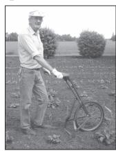
Mel Primrose fastened the handles off an old rototiller to the front wheel fork assembly of an old bicycle. Then he added a 16-in. wide, sharpened flat steel bar behind the wheel to do the weeding.
