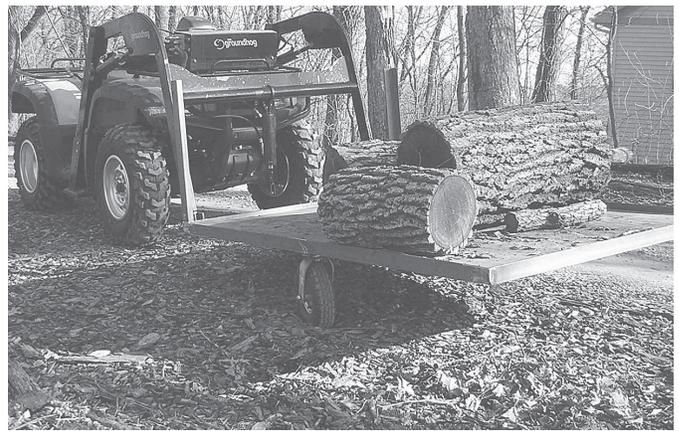
Trailer with caster wheels hooks onto ATV's loader arms (above). The operator simply lifts the loader arms to dump the load.
